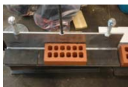
Figure 13. Left support of the lintel with neoprene layer between brick and steel.
