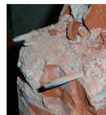
Figure 24. Shear failure of the 3 rd tested brick lintel (5 galva. B 500). Figure 25. View of collapsed lintel after testing: a) central crack; b) reinforcement detail.
