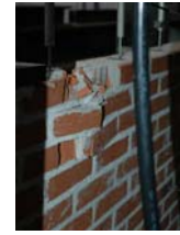
Figure 19. Failure due to horizontal compression of the 1 st tested brick lintel (2 inox. B 800). Figure 20. View of collapsed brickwork after testing: a) At the left jack; b) At the right jack.
