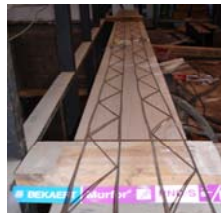
Figure 11. a) Continuous bed joint reinforcement; b) Murfor.5/S-80mm. 5.85m (inox. B800) Figure 12: Arrangement of extensometric gauges in 2 Murfor centre (B1, B2, B3, B4).
