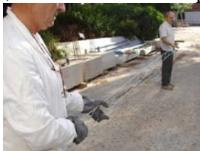
Figure 11. a) Continuous bed joint reinforcement; b) Murfor.5/S-80mm. 5.85m (inox. B800) Figure 12: Arrangement of extensometric gauges in 2 Murfor centre (B1, B2, B3, B4).
