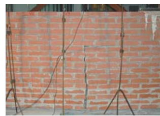
Figure 24. Shear failure of the 3 rd tested brick lintel (5 galva. B 500). Figure 25. View of collapsed lintel after testing: a) central crack; b) reinforcement detail.
