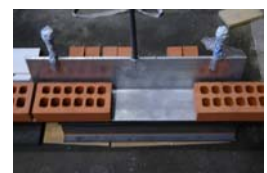
Figure 13. Left support of the lintel with neoprene layer between brick and steel.
