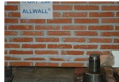
Figure 22. Type of shear failure of the 2 nd tested brick lintel (4 Inox. B 800). Figure 23. View of collapsed lintel after testing: a) left shear crack; b) right shear crack.
