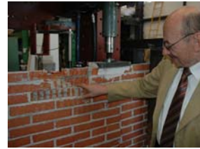
Figure 19. Failure due to horizontal compression of the 1 st tested brick lintel (2 inox. B 800). Figure 20. View of collapsed brickwork after testing: a) At the left jack; b) At the right jack.
