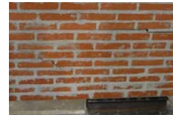
Figure 22. Type of shear failure of the 2 nd tested brick lintel (4 Inox. B 800). Figure 23. View of collapsed lintel after testing: a) left shear crack; b) right shear crack.
