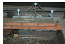
Figure 13. Left support of the lintel with neoprene layer between brick and steel.
