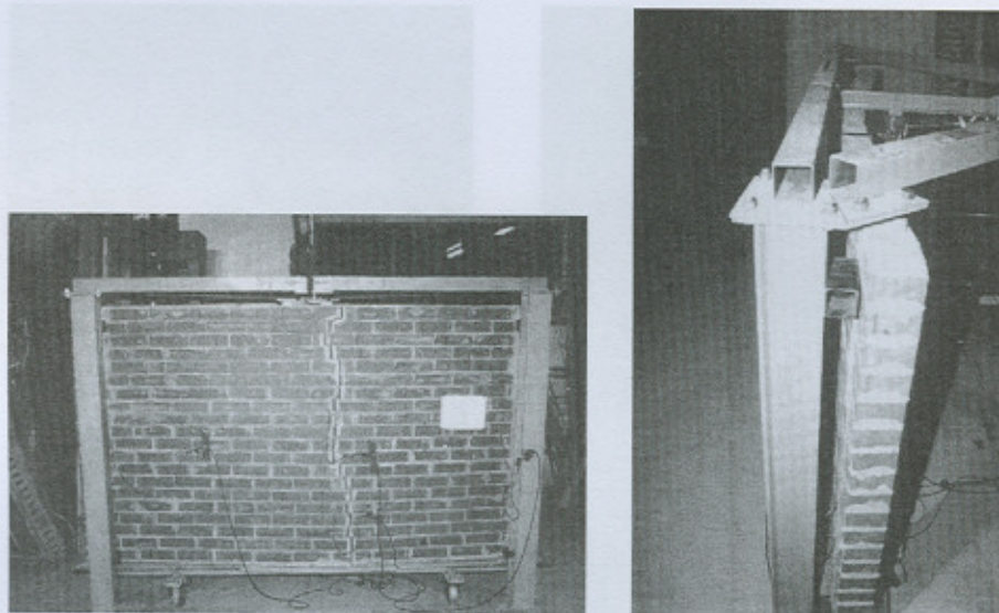
Figure 11. Front view of the Plate after testing with vertical crack in the middle third of the wall. Figure 12. Side view of the Plate after testing with breakage suffered by vertical failure
