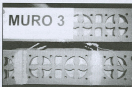
Figure 6. Tested specimen in which it is possible to observe the buckling of the diagonal reinforcement..
